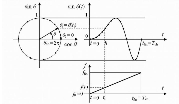
**Fig. 2.** Waveform genesis of a single-cycle linear sinusoidal chirp at  $f_0 = 0$  and  $\theta = 0$ .
