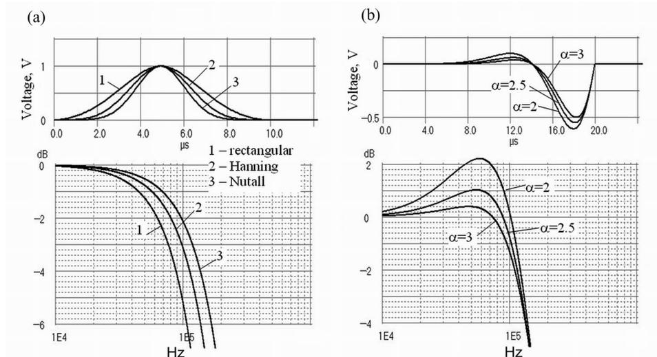
**Fig. 8.** Waveforms and RMS-SD of windowed titlets: (a) double quarter-cycle ( $L = 1/4$ ) linear titlet; (b) single-cycle ( $L = 1$ ) linear titlet, non-symmetric windowing,  $\alpha = \text{var}$ .
