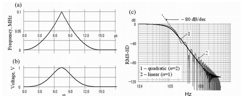
**Fig. 7.** Bidirectional (up-down) quarter-cycle quadratic titlet: (a) instantaneous frequency vs time; (b) normalized waveform; (c) normalized RMS spectral density.
