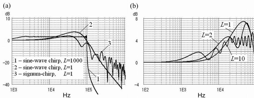
**Fig. 5.** Comparison of normalized RMS spectra: (a) sine-wave and signum-chirps; (b) sine-wave chirps with different number of cycles.
