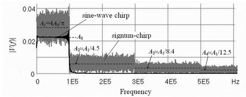
Fig. 4. Magnitude spectra of long linear chirps ( $L = 1000$ ).
