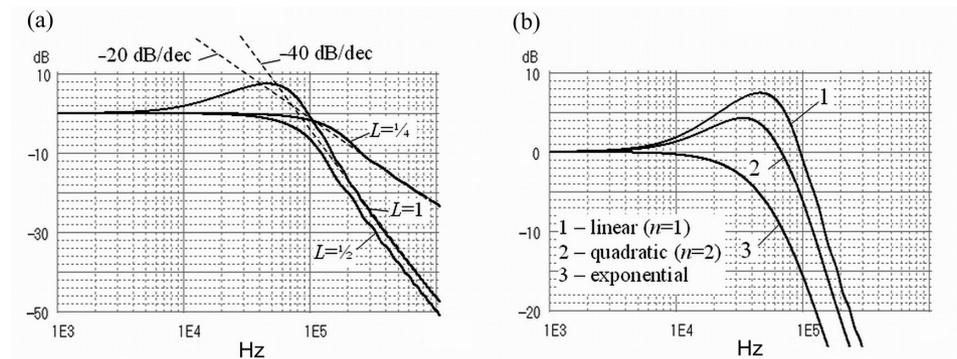
**Fig. 6.** Normalized RMS spectral density functions of sine-wave titlets with  $f_{fin} = 100$  kHz: (a) linear titlets,  $n = 1$ ,  $L = \text{var}$ ; (b) titlets of different type,  $L = 1$ .
