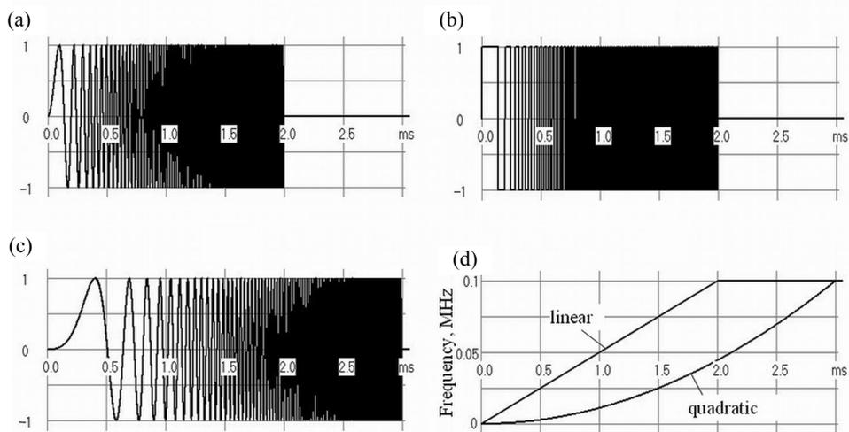
**Fig. 1.** Normalized waveforms vs time of a 100-cycle chirps with  $f_0 = 0$  and  $f_{fin} = 100$  kHz: (a) linear; (b) linear signum-chirp; (c) quadratic; (d) variation (linear and quadratic) of the instantaneous frequency vs time.
