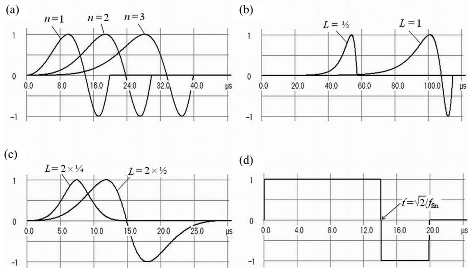
**Fig. 3.** Waveforms of typical titlets with  $f_0 = 0$  ( $f_0 = 1$  Hz for exponential chirp) and  $f_{fin} = 100$  kHz: (a) single-cycle sinusoidal power chirps; (b) single- and half-cycle sinusoidal exponential chirps; (c) bidirectional double quarter- and half-cycle sinusoidal quadratic chirps; (d) single-cycle signum-chirp.
