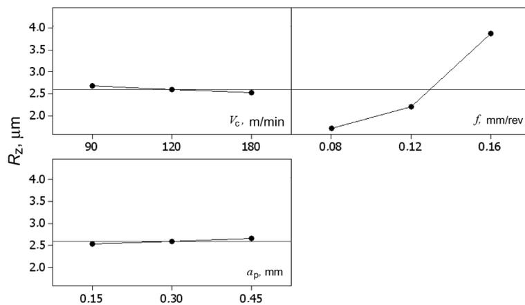
Fig. 7. Main effects plot for  $R_z$ .
