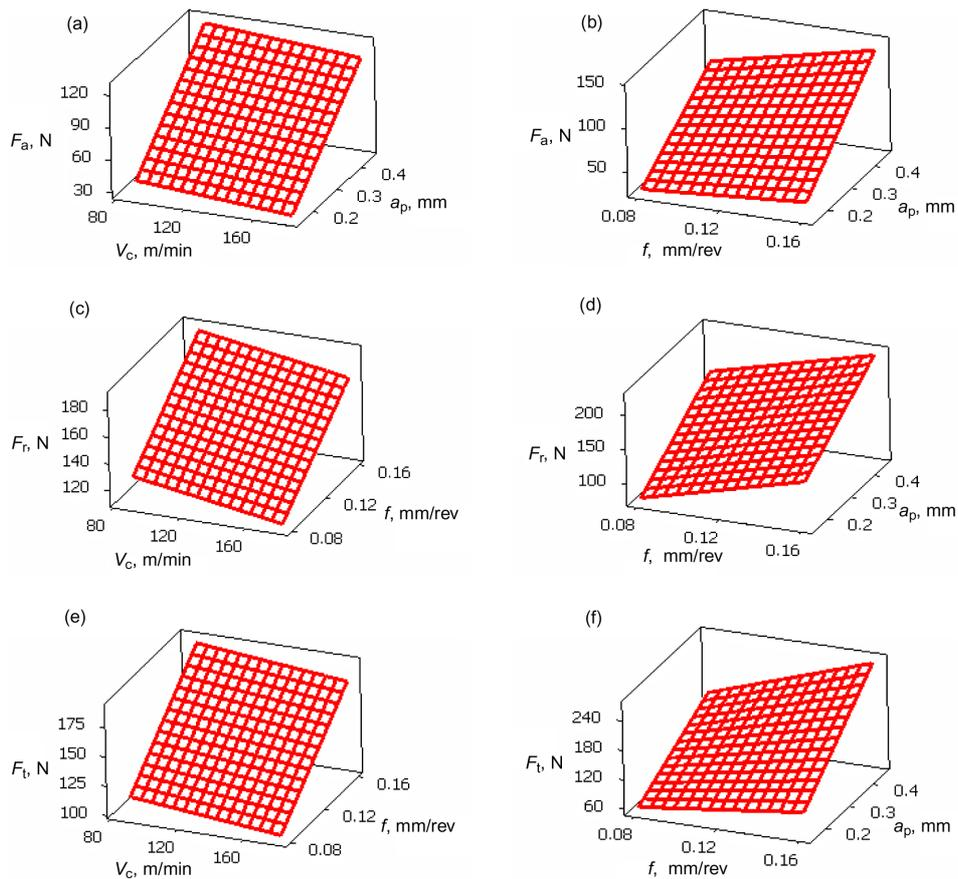
Fig. 4. 3D Surface plots of cutting forces.
