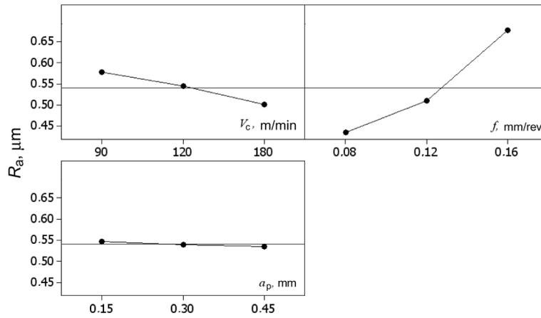
Fig. 5. Main effects plot for  $R_a$ .
