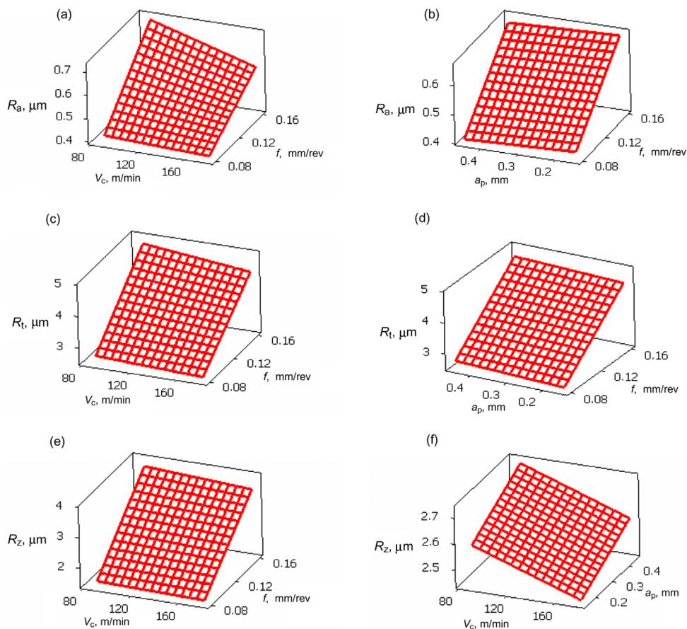
Fig. 8. 3D Surface plots of roughness.
