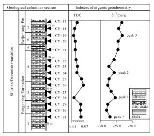
**Fig. 2.** Stratigraphic succession, total organic carbon content and stable isotopic ratio of organic carbon versus depth in the Changwantang Section.
