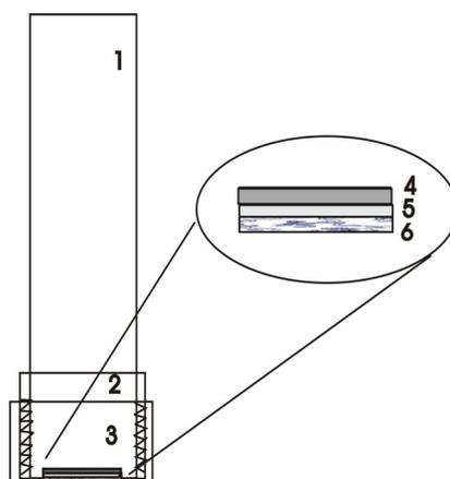
Fig. 1. Schematic drawing of the used BOD biosensor: 1 – sensor body, 2 – attached head-cap, 3 – threaded holder, 4 – cathode, 5 – Teflon film, 6 – membrane with immobilized bacteria.
