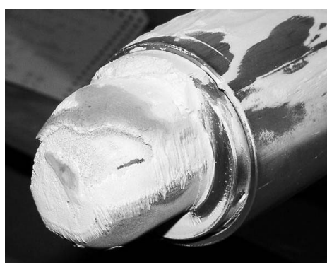
b) Probe tip after longer testing (~20 hours). Strongly moistened deposit accumulated on tip surface and probe sleeve.
