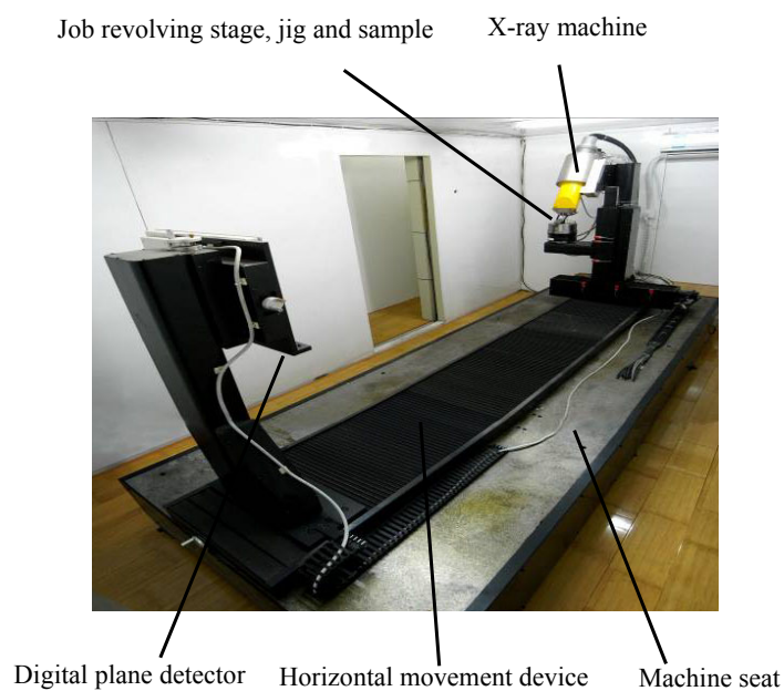
Fig. 1. Micro-CT experimental system.
