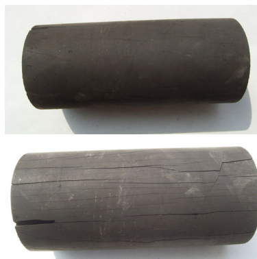
Fig. 4. Comparison of an oil shale sample before and after the permeability experiment.
