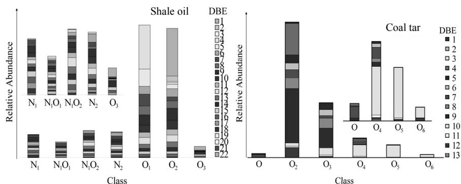
Fig. 2. Heteroatom class and type distribution of LSO and SLTCT derived from a negative-ion ESI FT-ICR MS spectrum.
