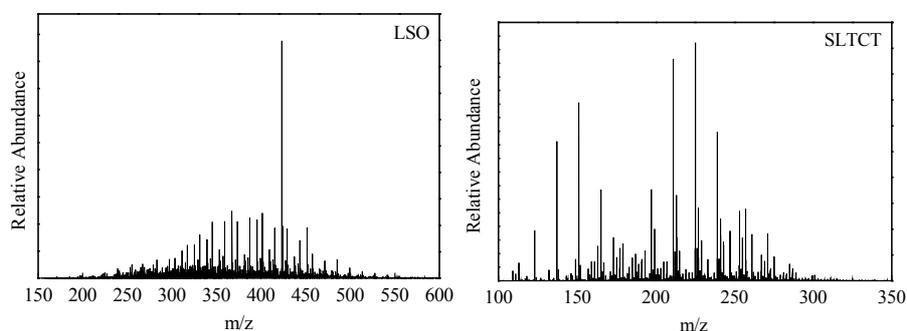
Fig. 1. Negative-ion ESI FT-ICR MS spectrums of LSO and SLTCT.
