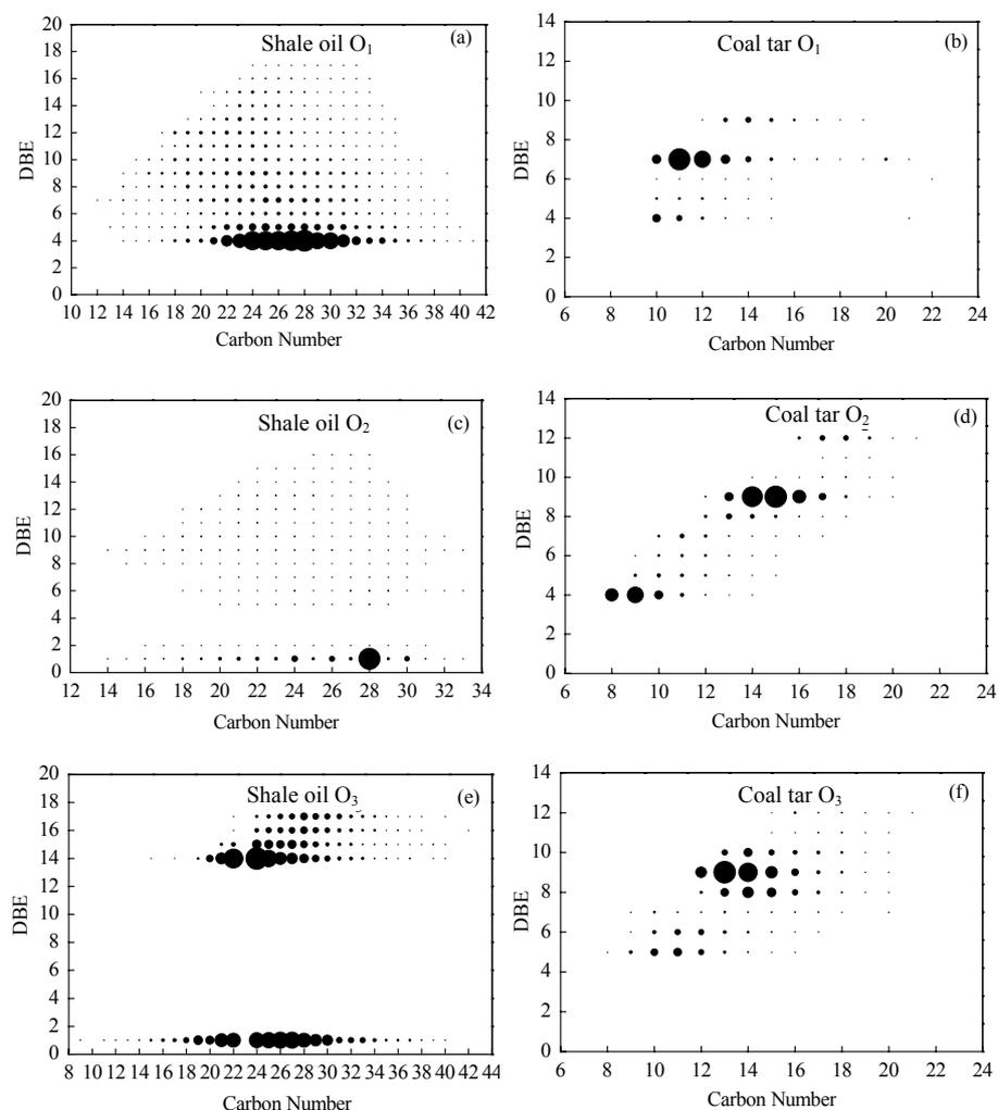
Fig. 3. Plots of DBE versus the carbon number of heteroatom compounds in LSO and SLTCT.
