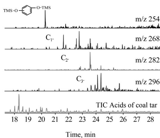
Fig. 5. Dihydroxybenzenes in the acid fraction of SLTCT.
