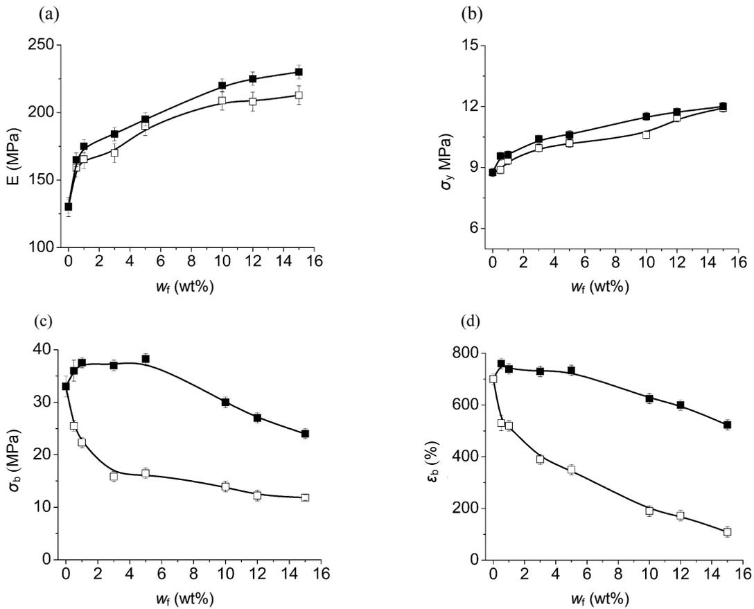
**Fig. 5.** Tensile modulus  $E$  (a), stress at yield  $\sigma_y$  (b), stress at break  $\sigma_b$  (c) and strain at break  $\epsilon_b$  (d) of EOC17 nanocomposites with MWCNTs (open symbols) and P3OT-f-MWCNTs (closed symbols).
