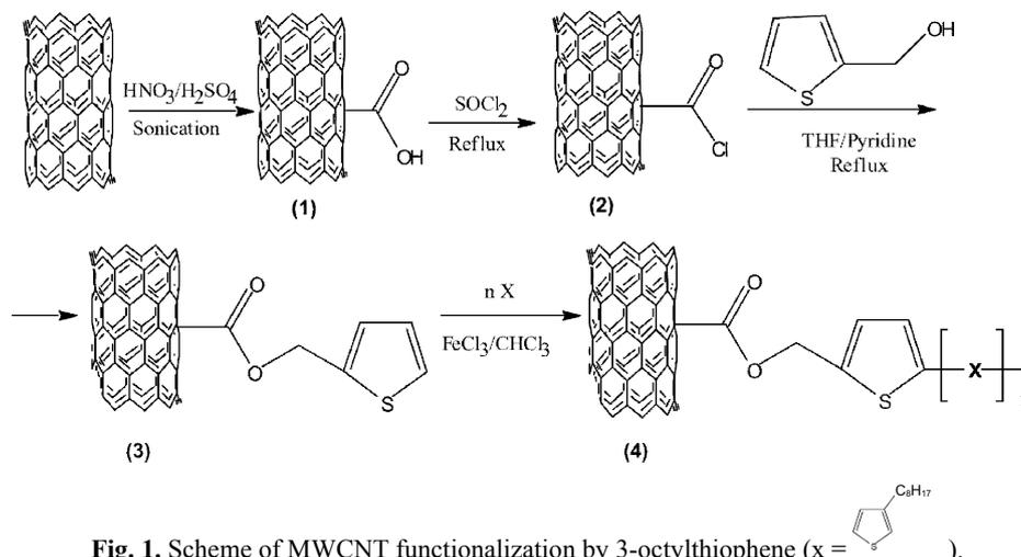
Fig. 1. Scheme of MWCNT functionalization by 3-octylthiophene ( $x =$
