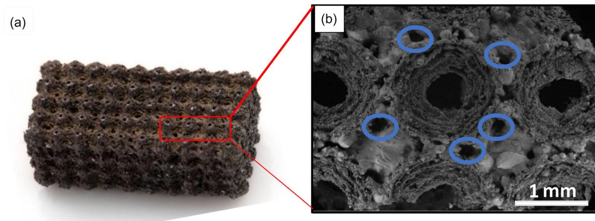
**Fig. 2.** As-synthesized  $\text{Si-CaSiO}_3$  scaffolds printed by selective laser melting (a) and the microstructure of the scaffolds with macropores ( $\sim 400 \mu\text{m}$ ) and mesopores (blue circles, pore size  $\sim 15\text{--}50 \mu\text{m}$ ) (b).
