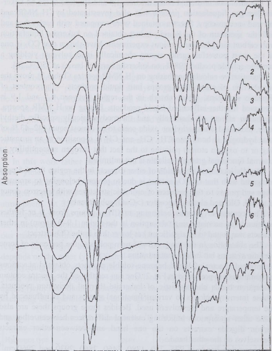
Fig. 2. Infrared spectra of the liquid products obtained on kukersite kerogen liquefaction in the following solvents: diethyl ether (1) and dioxane-1,4 (2) at 330 °C, ethylene oxide (3) at 300 °C, diethyl ether (4), dioxane-1,4 (5), ethylene oxide (6) and carbon dioxide (7) at 350 °C
