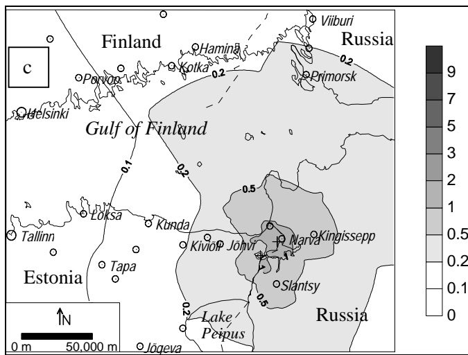
Fig. 3. Annual mean concentration of SO 2 in the surface layer of the atmosphere in the surroundings of Narva PPs, µg m -3 . Top-down: (a) during 1990–1991, (b) 2000–2001 and (c) after renovation of two power units. In calculations the following emission intensities of SO 2 with flue gases were used: in 1990–1991 – 6255–9170 g s -1 , in 2000–2001 – 4000–5530 g s -1 and after renovation of power units – 1890–3165 g s -1 .
