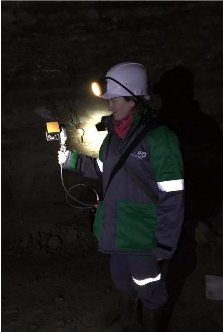
Fig. 2. The handheld laser scanner GeoSLAM ZEB-REVO in the oil shale mine.
