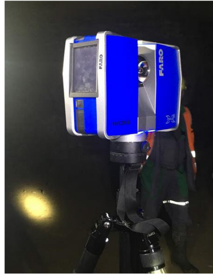
Fig. 3. The tripod mounted terrestrial laser scanner Faro Focus used for acquiring the reference data for the oil shale mine survey.
