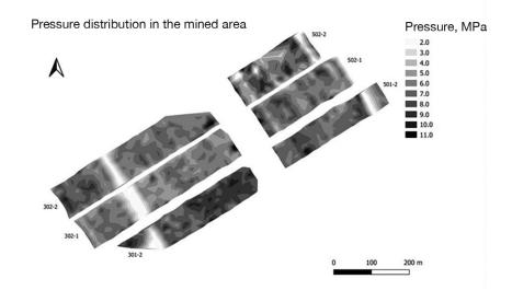
Fig. 2. Mapped distribution of pressure in the pillars (as an example). The darker is the colour, the higher is the pressure in the pillar.
