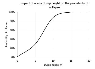
Fig. 5. Impact of the waste dump height on the probability of rooms collapse (illustrative).
