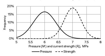
Distribution of the pressure and bearing capacity of pillars
