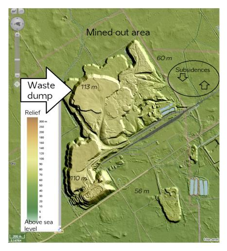
Fig. 1. Enrichment waste dump of Estonia mine on the mined-out area. The level of the mine horizon is from -10 to +10 m above sea level. Source: https://xgis. maaamet.ee/maps/XGis?app\_id=UU82A&user\_id=at&LANG=2&WIDTH=118 2&HEIGHT=851&zlevel=7,693695.3125,6567830.078125&setlegend=SHYBR\_ALUS01\_82A=0,SHYBR\_ALUS11\_82A=1
