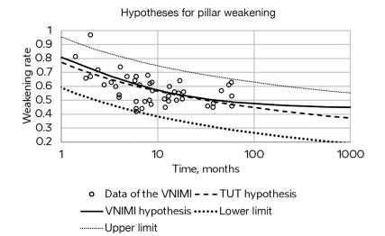
Fig. 4. Two hypotheses for the weakening of pillars as a result of oil shale creep.
