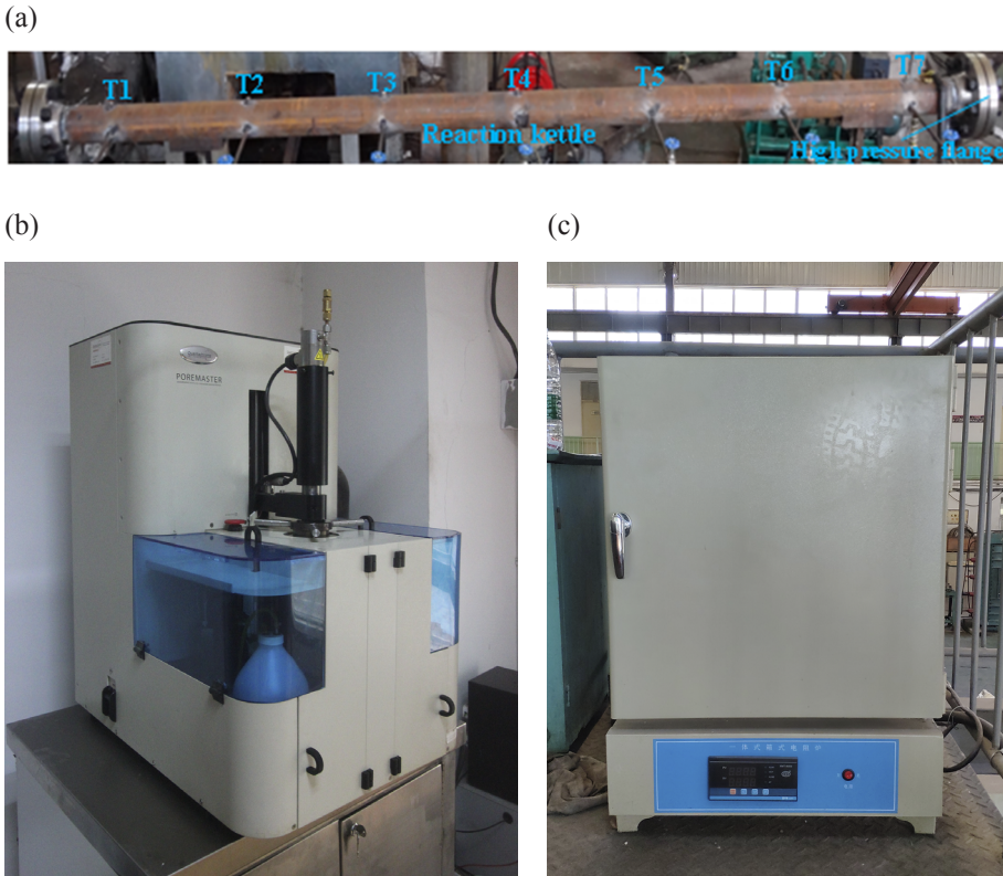
Fig. 1. Schematic diagram of test equipment: a) long airway reactor, b) mercury porosimeter, c) muffle furnace.
