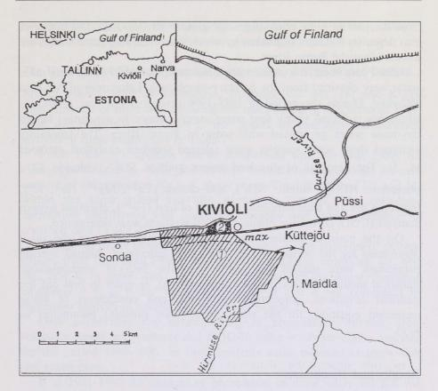
Sketch map of closed *Kiviõli* mine region: 1 - mined area, 2 - pit bottom area under the territory of *Kiviõli* OSP; -- - maximum level of water flux in mine galleries (41.5 m abs.)
