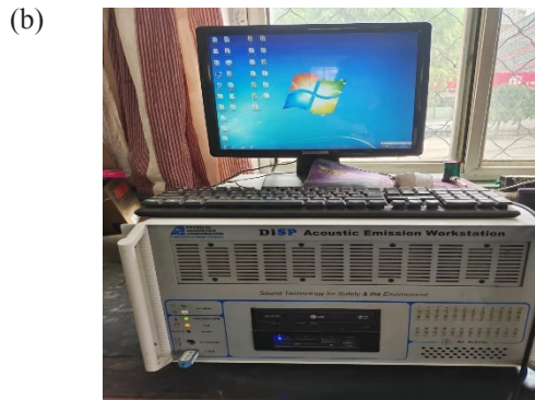
Fig. 2. (a) Schematic of the acoustic emission detection process; (b) the PCI-2 device.
